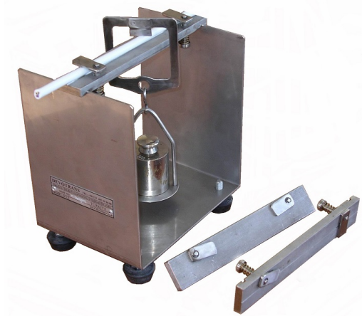
DVT KBS – Equipment for pressure test under high temperature
